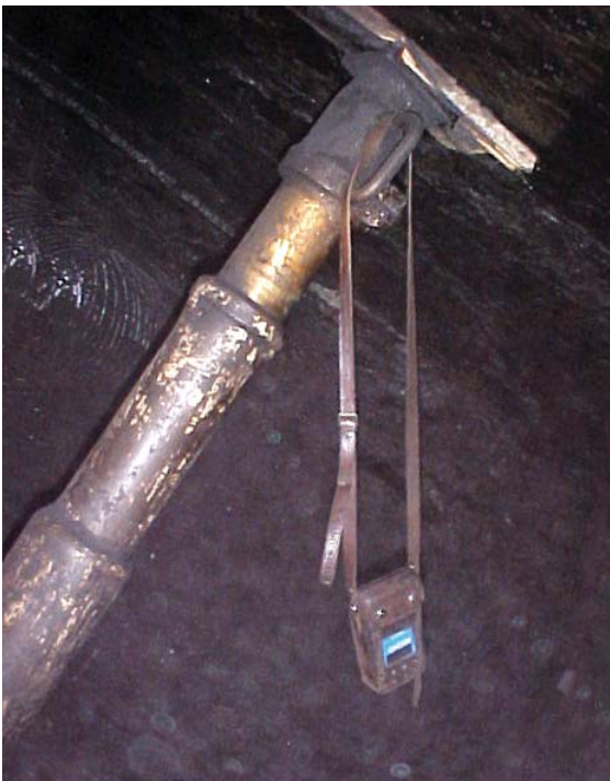
A Penny Duke Prop supporting a long wall at 30° inclination
